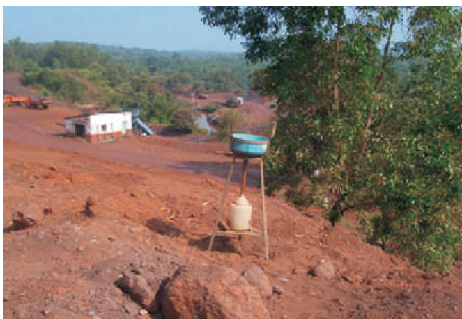
Dust fall apparatus used to measure dustfall at Goa Iron ore mines.
